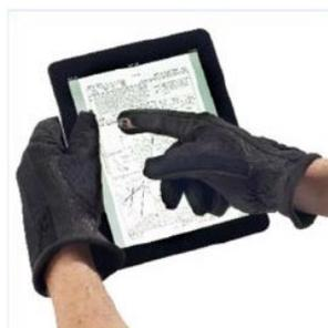
Some gloves are designed with conductive material sewn into the fingertips so they can be used with a touchscreen but the material on the rest of the hand will not be conductive. Alternatively, you could use a pair of gloves and cut off the glove fingertips of the fingers you are wanting to use on the touchscreen.
