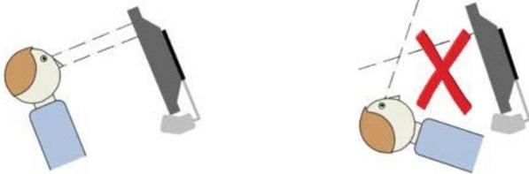
Positioning for eye gaze is extremely important. The goal when positioning for eye gaze use is to achieve a stable eye image for the eye gaze device to track. The eye gaze system should remain parallel with the student's head. This means if the student is reclined the eye gaze should be positioned above them. A certain distance needs to be maintained between the user and the device. Each device will have its own recommendations, however the distance required is usually between 45cm and 85cm.
